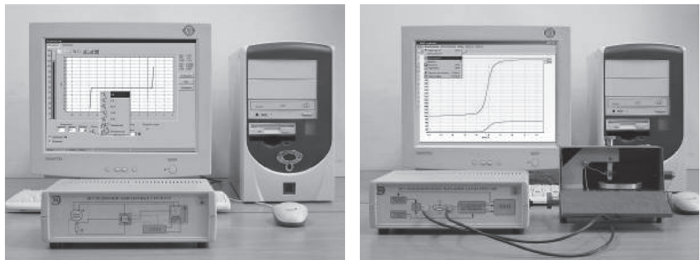
Fig. 3. Automated Complexes for Measuring Volt-Ampere (a) and Voltage-Capacitance Characteristics (б) of Microsystems
